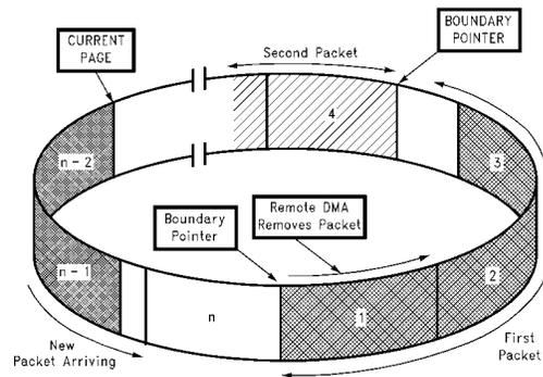
FIGURE 39. 1st Received Packet Removed by Remote DMA
