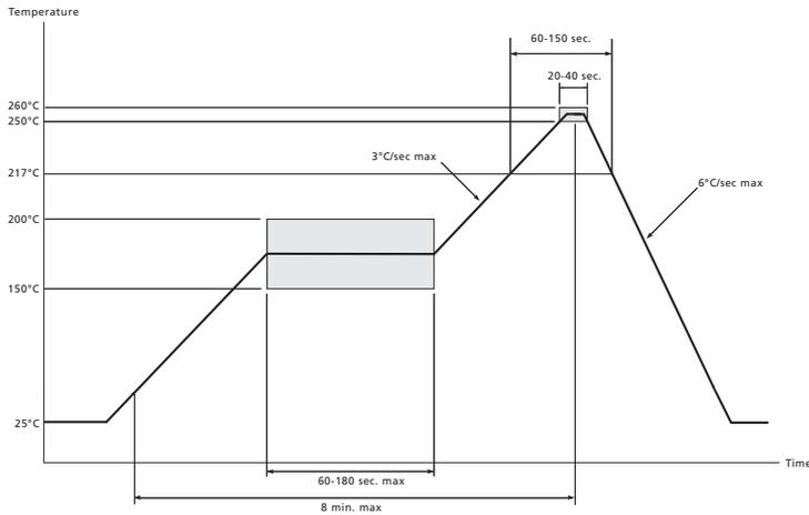
Figure 6-3: Maximum Pb-free Solder Reflow Profile (Preferred)
