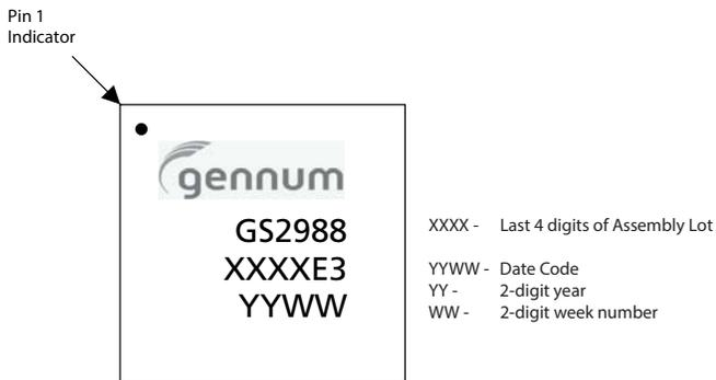
Figure 6-4: Marking Diagram
