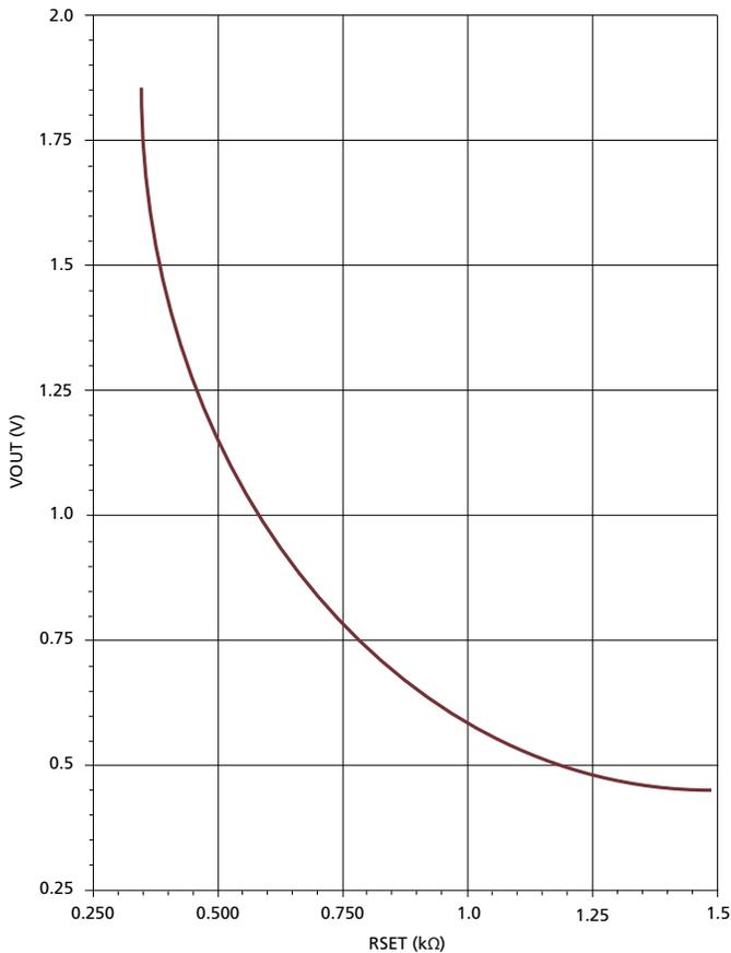
**Figure 4-1: V<sub>OUT</sub> vs. RSET**
