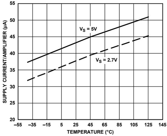
Figure 33. Supply Current per Amplifier vs. Temperature
