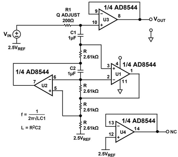
Figure 38. FDNR 60 Hz Notch Filter with Output Buffer
