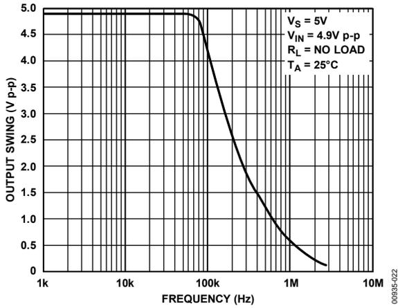
Figure 23. Closed-Loop Output Voltage Swing vs. Frequency,
