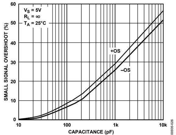
Figure 27. Small Signal Overshoot vs. Load Capacitance
