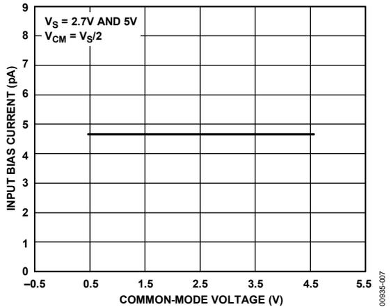
Figure 7. Input Bias Current vs. Common-Mode Voltage
