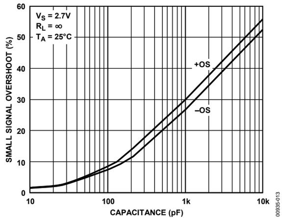
Figure 13. Small Signal Overshoot vs. Load Capacitance
