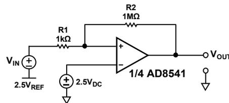
Figure 39. AD854x Comparator Application—Overload Detector
