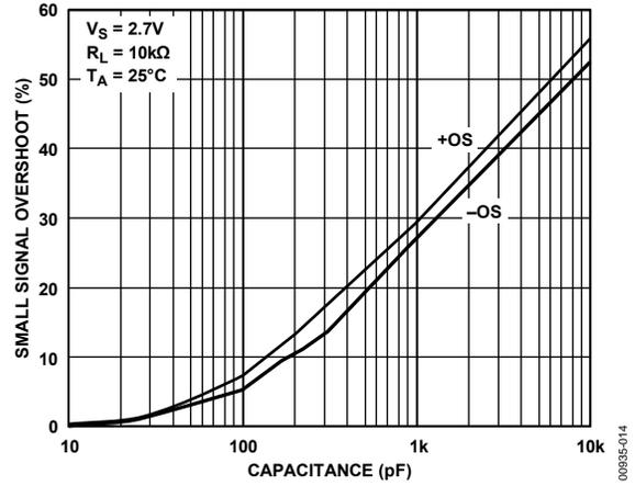
Figure 14. Small Signal Overshoot vs. Load Capacitance
