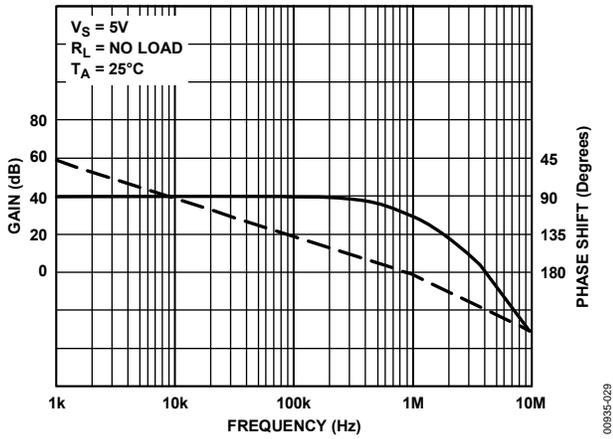
Figure 30. Open-Loop Gain and Phase vs. Frequency
