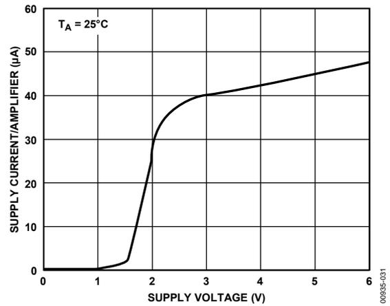
Figure 32. Supply Current per Amplifier vs. Supply Voltage
