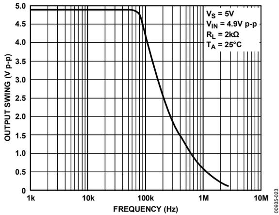
Figure 24. Closed-Loop Output Voltage Swing vs. Frequency
