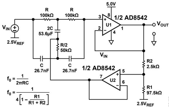
Figure 36. 60 Hz Twin-T Notch Filter, Q = 10
