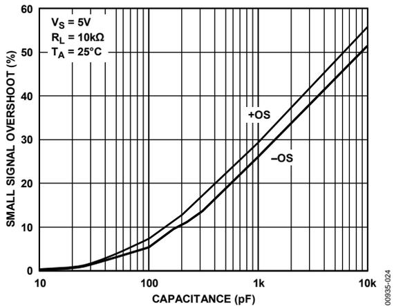
Figure 25. Small Signal Overshoot vs. Load Capacitance
