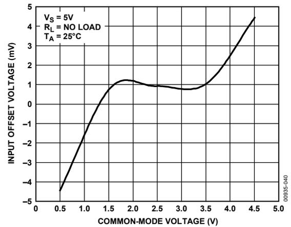
Figure 21. Input Offset Voltage vs. Common-Mode Voltage
