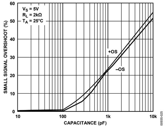
Figure 26. Small Signal Overshoot vs. Load Capacitance
